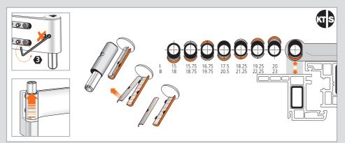
Adjustment of sealing pressure within upstand range.
